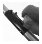
**NOTE:** Whilst inserting the shaft into the joining clamp the lower shaft may need to be rotated a bit so the internal shaft components can engage correctly.
